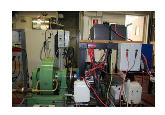
Basically, it's composed of a battery pack, an inverter, an electric synchronous motor, a control system, a transmission system, blocks of resistive forces and tables of reference data.
